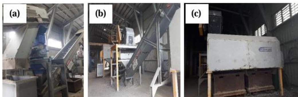
Fig.1. Waste glass processing stage. a- Mil-tek GC600 Glass Crusher, b- Retsch AS 200 Vibratory Sieve Shaker, c- IKA MF 10 Basic Analytical Mill
