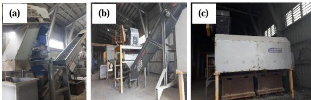
Fig.1. Waste glass processing stage. a- Mil-tek GC600 Glass Crusher, b- Retsch AS 200 Vibratory Sieve Shaker, c- IKA MF 10 Basic Analytical Mill
